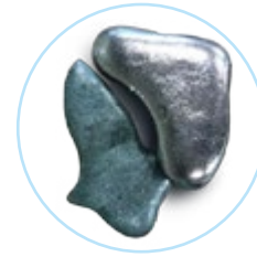
Slag with concentrated rare earths (left) and pig iron.
